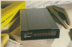
X25 PAD. The letters PAD stand for Packet Assembler/Disassembler.
